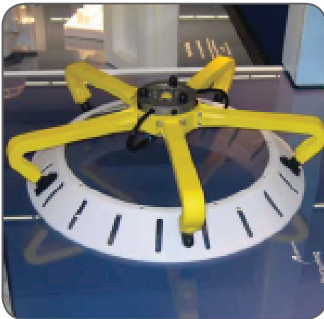
Figure 1: Components for this robotic gripper were first prototyped, then manufactured, using FDM (Fused Deposition Modeling).
