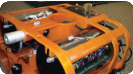
Figure 2 and 3 : University of Central Florida Electronics enclosure. The frame was first prototyped, then manufactured from ABSi using the same FDM system
